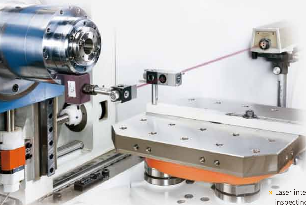
» Laser interferometer is used for inspecting indexing degree
