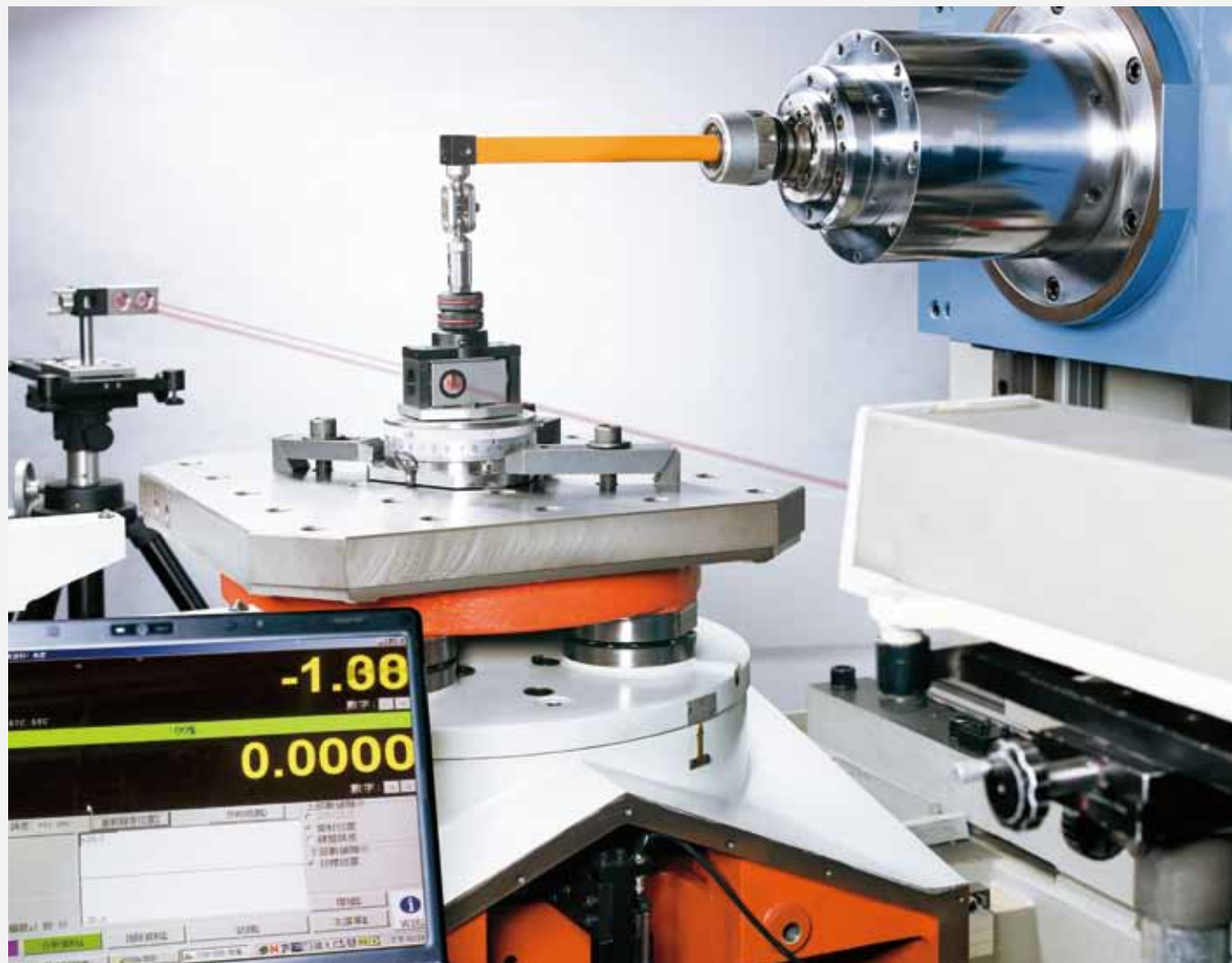
» Laser interferometer is used for inspecting indexing degree
